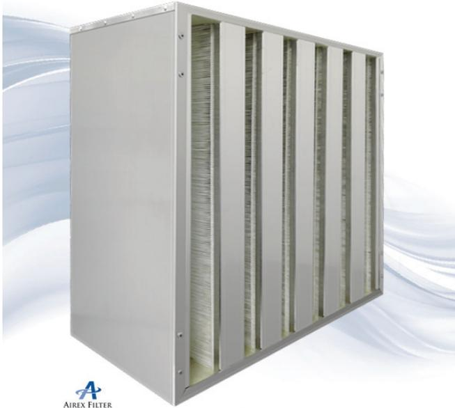
The Airex Filter SuperFlow 24 is a V-bed HEPA filter (99.99% at 0.30 micrometer) specifically designed for high airflow applications requiring HEPA efficiency at an ultra low-pressure drop. The SuperFlow 24 can be incorporated into systems with air velocities of 600 fpm and a pressure drop of 1° w.g.
